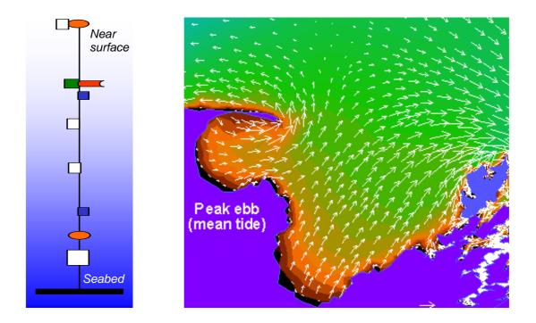
Data from instrument moorings provide calibration for computer circulation simulations – a cornerstone for understanding and predicting the physical and biological properties of these Bays. Instruments on the moorings measure temperature, salinity, tide height and currents. The computer simulation shows the interaction between Golden Bay, Tasman Bay and Cook Strait waters during the change between high and low tide.
